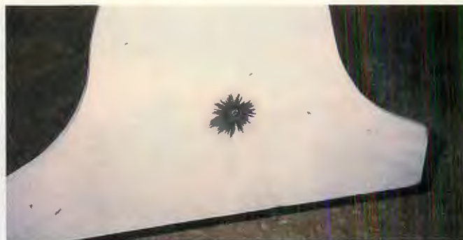
Only a tiny smear of metal results from the impact of a round of .30-06 GI Ball at 50 yards. No damage was done from 100 yards.
